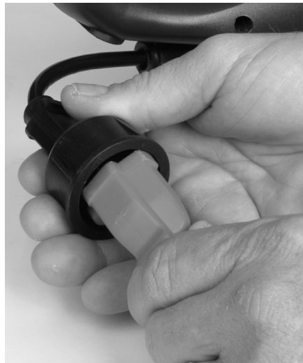
Figure 3-1: Plugging trimmer power cord into extension cord
